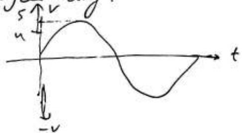
angular measurement of sine wave
