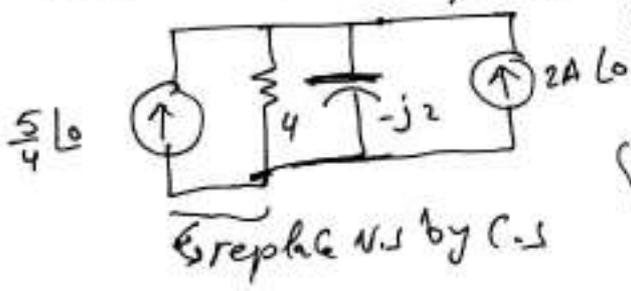
Coil removed has no effect with independent source
