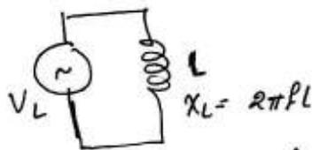
$Z = \frac{V_L L_0}{I_L L_0} = \frac{X_L L_0}{L_0} = jX_L = j\omega L = j2\pi fL$
