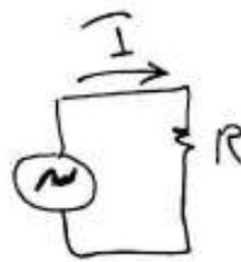
During (+ve half Cycle) → Voltage source is positive & current generates (clockwise)
