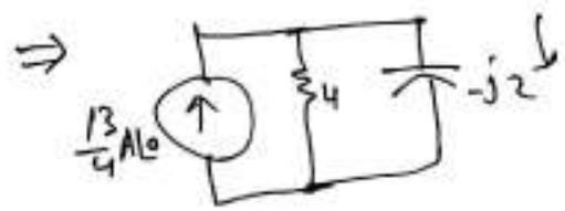
$$I = \frac{\frac{13}{4} \angle 0 \times 4}{4 - j2} = \frac{13 \angle 0}{4.47 \angle -26.56^\circ} = 2.9 \angle 26.56^\circ$$
