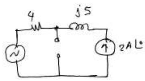
a) to calc  $Z_{th}$  (o.c. current source, s.c. voltage source)
