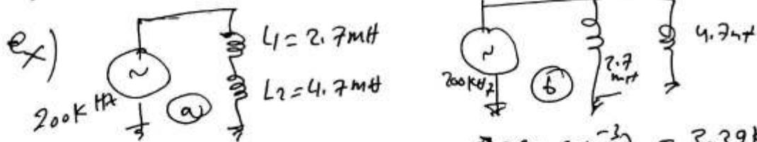
$$X_{L1} = 2\pi fL_1 = 2\pi \times (200 \times 10^3) \times (2.7 \times 10^{-3}) = 3.39 \text{ k}\Omega$$
