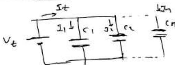
but  $V_T = V_1 = V_2 = \dots = V_n$
