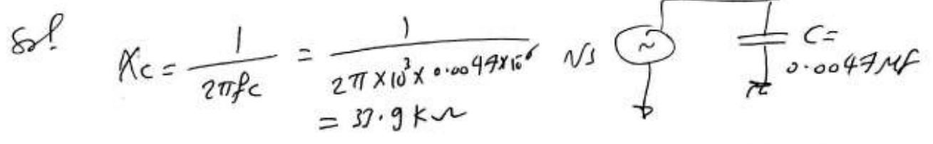
(a) Find the total capacitive reactance of the circuit
