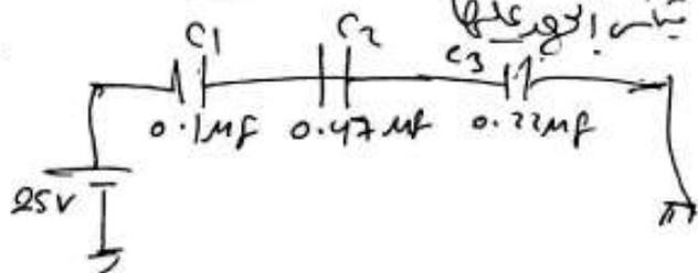
$$V_1 = V_T \frac{C_T}{C_1} = 25 \times \frac{0.06 \mu\text{F}}{0.1 \mu\text{F}} = 15\text{V}$$
